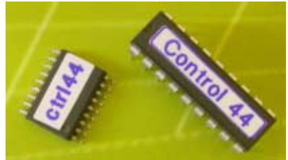
Figure 1: Control44 in SO, DIL packages
